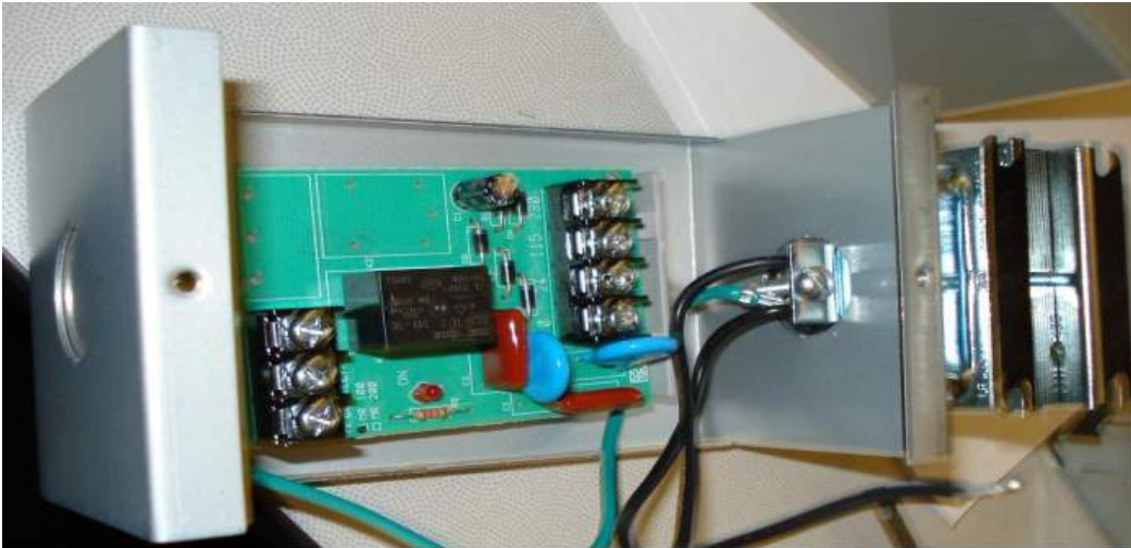
Figure 2: Model 592 transformer mounted onto an MR-101
